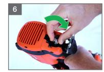
Carefully align fuel adaptor and cell stem
