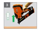
Allow recoil, work contact is released
