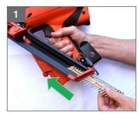
Slide nail strip into back of Magazine
